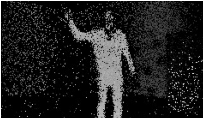
Fig. 7. Depth map output from time of flight camera
