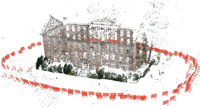
Fig. 4. Example Bundle Adjustment Output from Colmap
