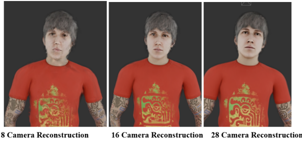
Fig. 2. Comparison of Reconstruction Quality with Increased Capture Density
