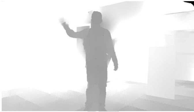
Fig. 8. Depth map output from stereo camera
